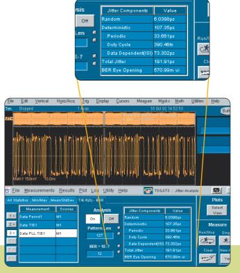
Figure 3. 2.5 Gb PLL TIE Rj/Dj with detail.
