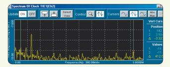
Jitter spectrum of the time trend plot. Harmonics of the triangle source are clearly defined.
