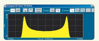
Jitter histogram of the result of the TIE of the above signal modulated by a sine wave, with a peak-to-peak value of about 100ps.
