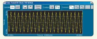
Jitter Time Trend. The pattern of jitter variation becomes apparent, and its correlation with one of several possible sources of coupled noise can be derived. The random component can still be seen as noise added to the sinusoidal modulation.
