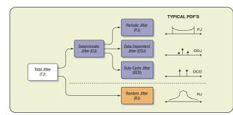
Figure 2. The jitter model first separates the total jitter (TJ) into random jitter (RJ) and deterministic jitter (DJ). The deterministic jitter is further subdivided into periodic jitter (PJ), duty-cycle dependent jitter (DCD), and data-dependent jitter (DDJ).
