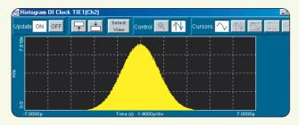
Jitter histogram for a Time-Interval Error (TIE) measurement. The continuous variable is mapped into 500 bins. The mean value is 0 nsec and the distribution is approximately Gaussian with a standard deviation under 1ps.
