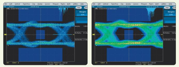
► Two masks - with one thousand hits (left) and one million hits (right) - showing the increase in peak-to-peak jitter over time. These also demonstrate DPX<sup>™</sup> technology acquiring more than 200K waveforms per second, with several measurements enabled.
